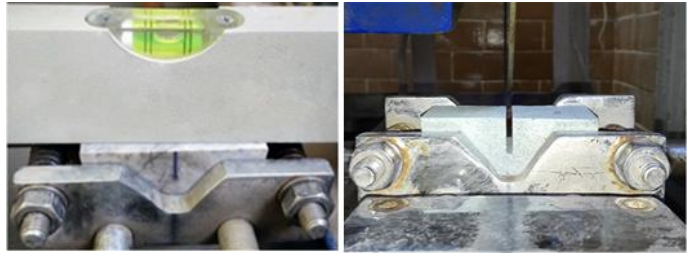
Figure 5. Notching the rock specimens
